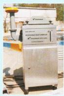
Hi – Volume Air Sampler For the monitoring of ambient air quality
